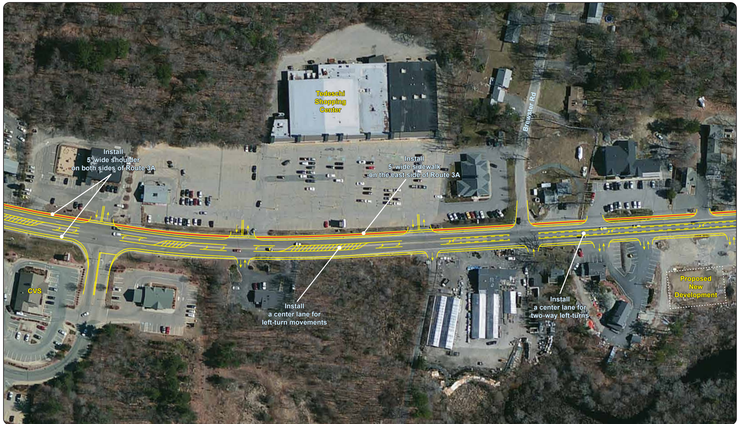
FIGURE 16 Proposed Long-Term Improvements Conceptual Plan Route 3A South Section (2)
