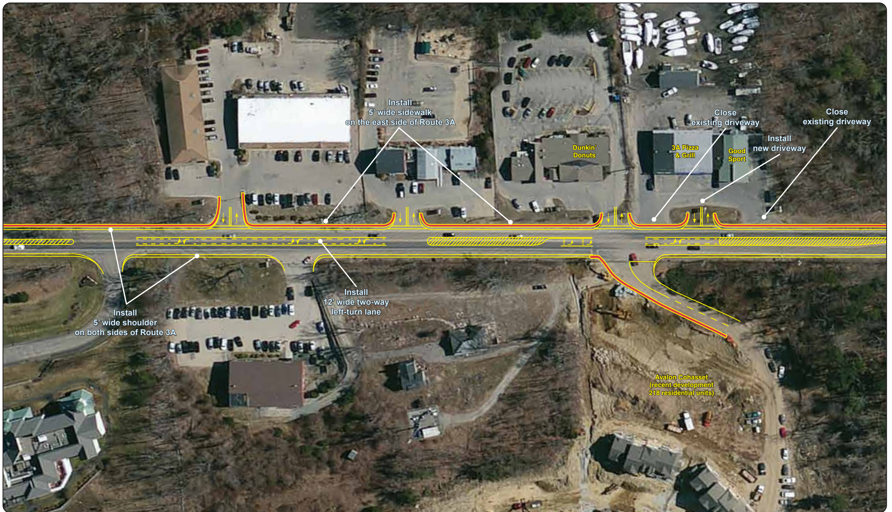
FIGURE 11 Proposed Long-Term Improvements Conceptual Plan Route 3A North Section (1)
