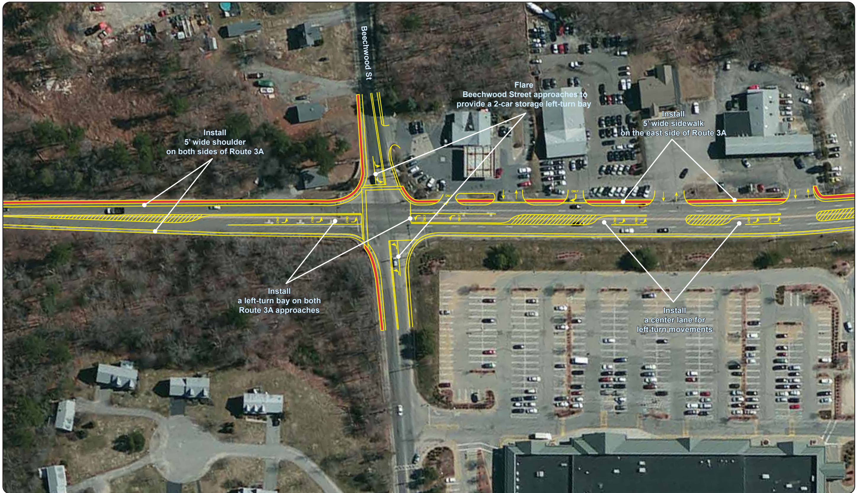
FIGURE 15 Proposed Long-Term Improvements Conceptual Plan Route 3A South Section (1)
