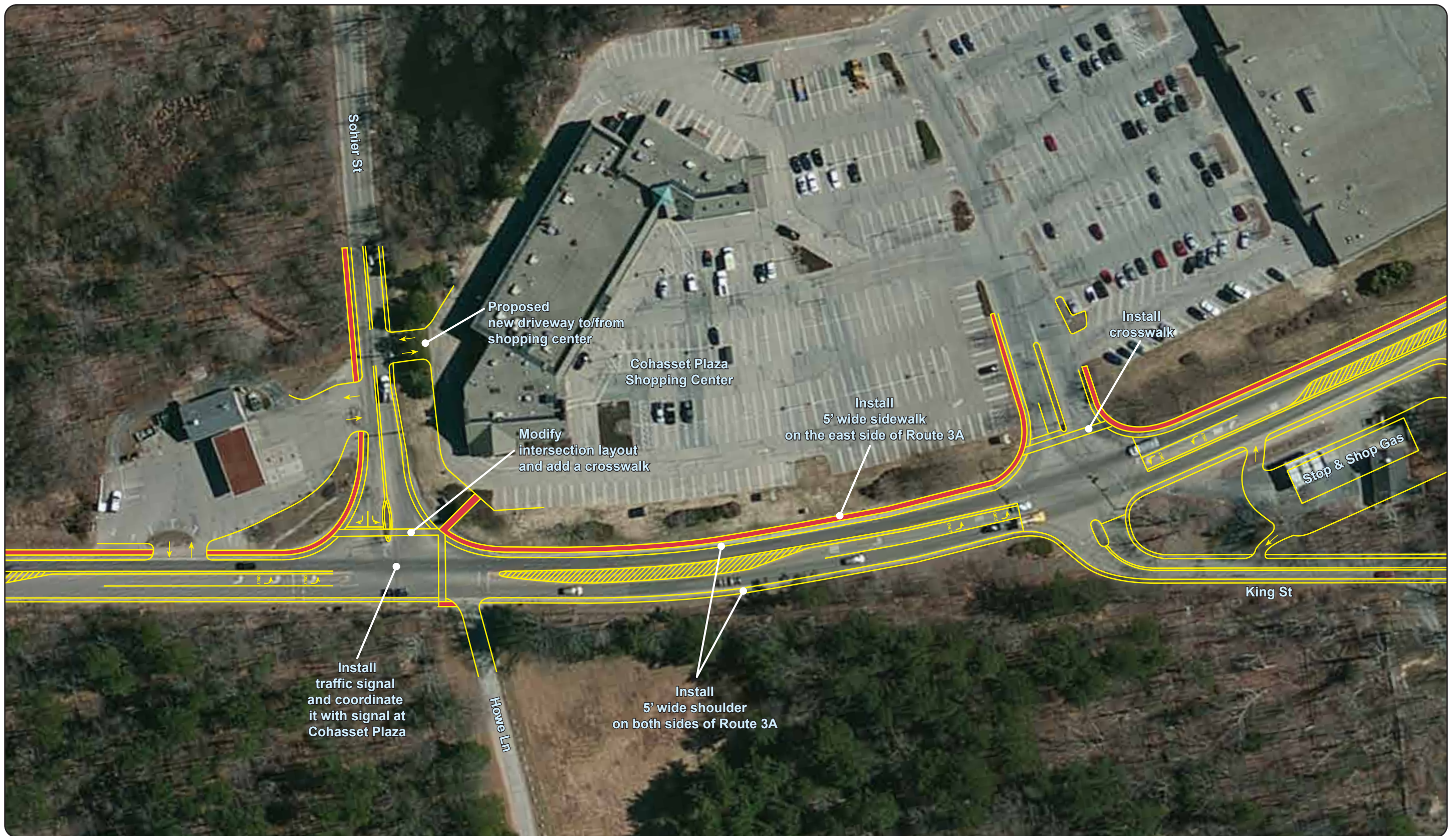
FIGURE 12 Proposed Long-Term Improvements Conceptual Plan Route 3A North Section (2)
