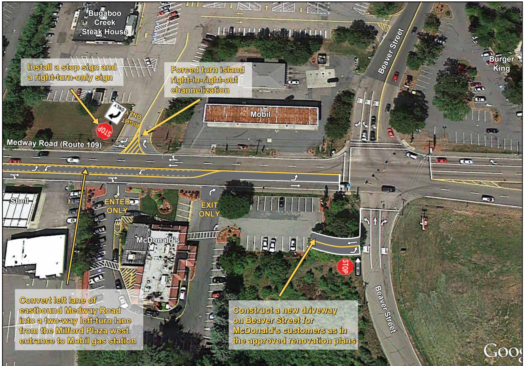
FIGURE 7 Alternative 2—Convert the Medway Road Eastbound Left Travel Lane into a Two-Way Left-Turn Lane
