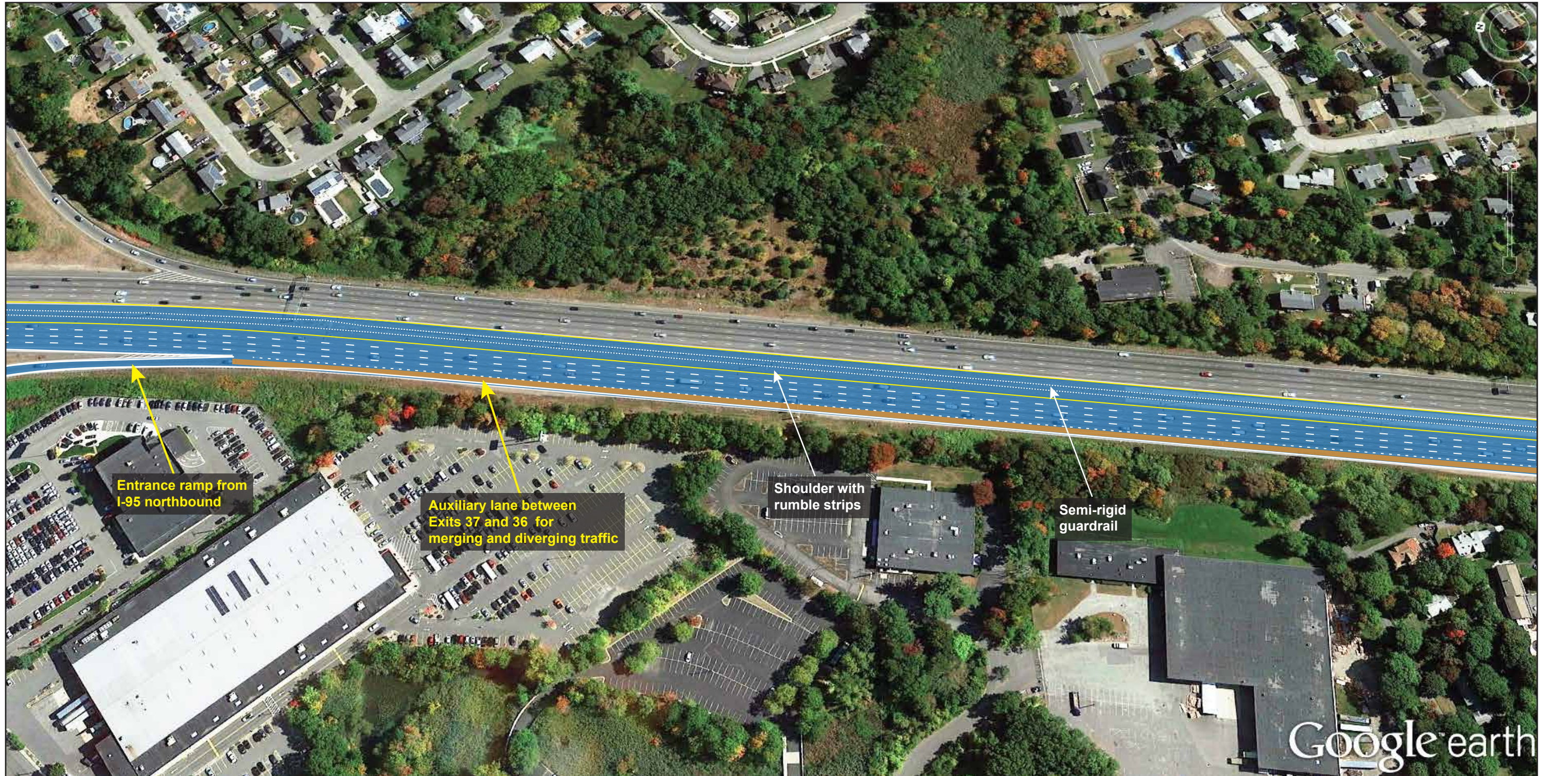
FIGURE 7 (Section 1) I-93 Southbound Segment: Between I-95 and Montvale Avenue Alternative 2: Construct an Auxiliary Lane Using Existing Right Shoulder
