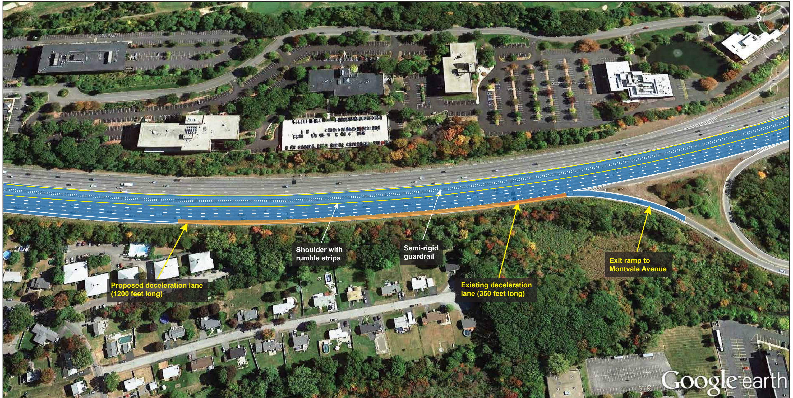
FIGURE 6 I-93 Southbound Segment: Between I-95 and Montvale Avenue Alternative 1: Lengthen Existing Deceleration Lane
