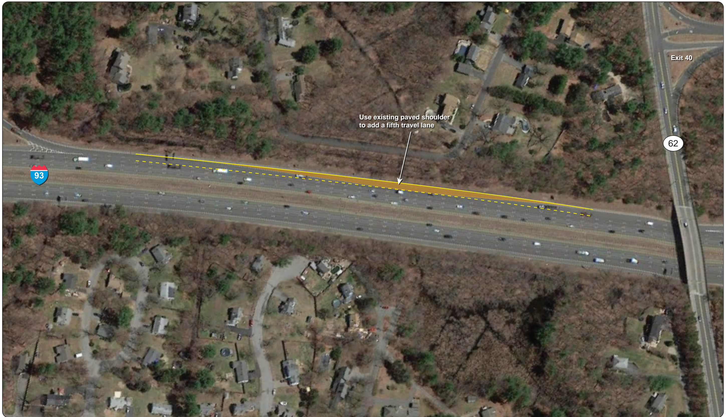
Figure 5 Location 1—I-93 Northbound between Exit 40 (Route 62) and Exit 41 (Route 125): Alternative 1—Create Auxiliary Lane
