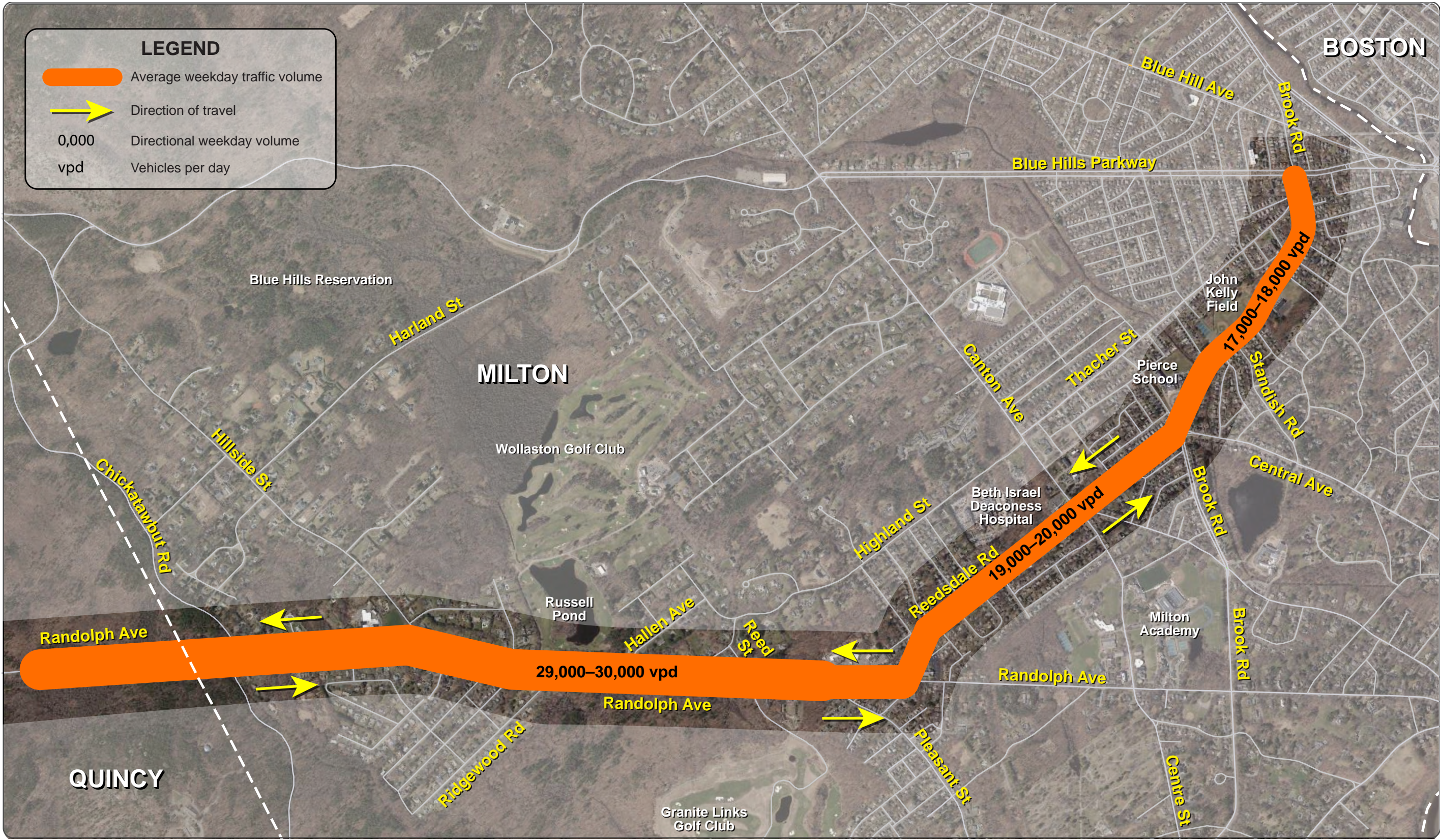
BOSTON REGION MPO Figure 4 Average Weekday Traffic Volumes Addressing Priority Corridors from the LRTP Needs Assessment: Route 28 Priority Corridor Study: Milton, Massachusetts
