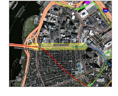
The proposed Red Line/Blue Line Connector consists of an extension of the MBTA Blue Line under Cambridge Street to the Red Line station at Charles/MGH. As currently envisioned, the project consists of two major components: (1) a new tunnel extending the Blue Line under Cambridge Street from Government Center to Charles Circle and (2) a new underground Blue Line station connected to the existing Charles/MGH Station. The project will also consider whether and how to relocate Bowdoin Station.
