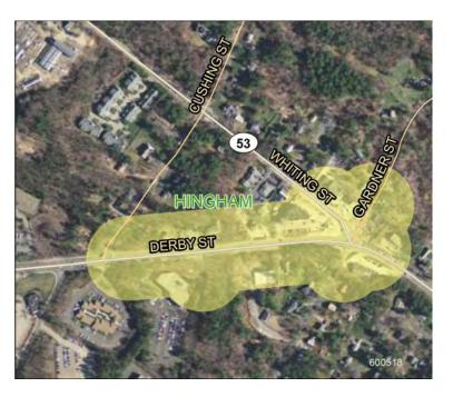
Work on this project will consist of intersection improvements at Derby Street, Whiting Street (Route 53) and Gardner Street. Work includes the installation of a new traffic signal system and geometric modifications at the intersection, including left turn lanes on Derby Street. The project extends to the Cushing Street intersection and will also provide a turn lane at Recreation Park Road. The project will also include improved accommodation for bicycles and pedestrians.
