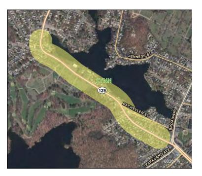
This roadway and safety improvement project includes drainage improvements, curbing, new sidewalks, wheelchair ramps, intersection improvements, pavement markings, signing, landscaping, and other incidental work. Project limits are from Colonial Avenue to about 150 feet south of Floyd Avenue (between Floyd and Cowdrey Road). The total project length is approximately 0.72 miles.
