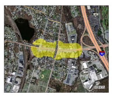
This project will widen Montvale Avenue to 4 lanes and provide turning lanes at Washington Street. New traffic signals will be installed along with new sidewalks, wheelchair ramps and new roadway pavement
