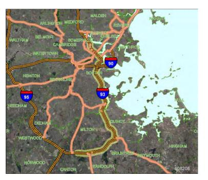
I-93 SE Expressway interstate maintenance resurfacing is proposed with a preservation treatment or thin bonded overlay to extend the pavement service life and improve safety.
