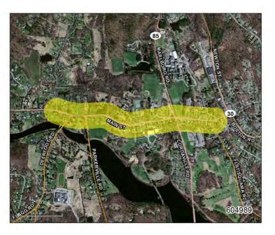
The purpose of this project is to reconstruct Main Street in Southborough with the intent to create a consistent roadway width. A continuous sidewalk will also be constructed along the southern side of the project. The intersection of Main Street (Route 30) and Marlborough Street/Cordaville Road (Route 85) are proposed to be realigned to include a new traffic signal system and left turn only lanes.
