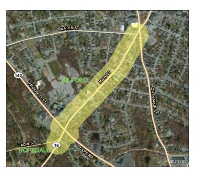
The project involves resurfacing along Route 16, from Water Street to just west of the Hopedale Town line, a distance of 0.6 miles. Additional work includes sidewalk reconstruction, culvert repairs and related work. The project includes improvements to the intersection of Route 16 and Route 140, including upgraded signal equipment and widening where feasible.
