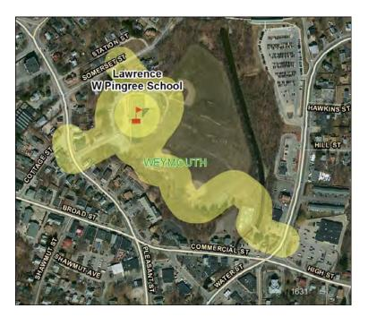
This project includes mill and overlay along Commercial Street from 500 ft north of Cottage Street to approximately 350 ft south of the school driveway. Pedestrian improvements will include wheelchair ramp and sidewalk reconstruction to meet ADA requirements. The curb bump out will narrow the roadway and reduce crossing distance. Share the road signs will be constructed.
