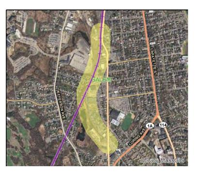
The project will construct 0.6 miles of shared off road path closing the gap between the existing Marblehead Rail Trail and the shared use path constructed along side Canal Street to Mill Street. The path will be 10 feet wide with 2 foot shoulders. The project includes the relocation of a railroad spur.
