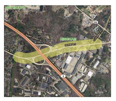
This project is proposed to address ongoing safety and capacity issues at the Derby Street/Route 3 ramps. Ramp modifications including signalization of ramps are proposed. In addition, there is a need to provide improved multi-modal accommodation on this targeted segment of Derby Street.
