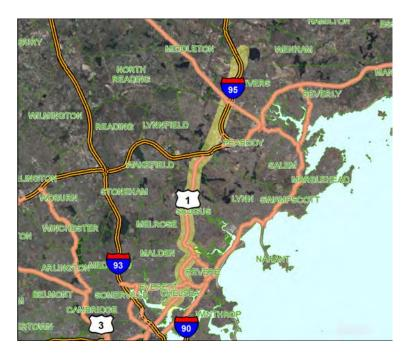
The project will consist of replacing guide and traffic signs, and supports, on Route 1 between the Tobin Bridge in Chelsea and Interstate 95 at the Danvers/Topsfield town line, including applicable signing on intersecting secondary roads. To ensure continued driver safety, new signs and supports meeting current retroreflectivity and design standards will be provided.
