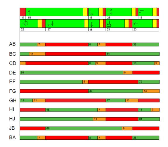
Average delay for all the crossings is shown in the body of the report. Here is an example output from the program used to determine pedestrian delay, applied to crossing the north leg of the intersection.
