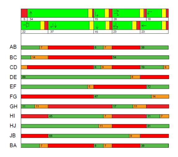
Average delay for all the crossings is shown in the body of the report. Here is an example output from the program used to determine pedestrian delay, applied to crossing the north leg of the intersection.
