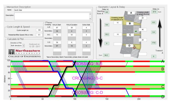
Report from the Northeastern University Ped/Bike Crossing Delay Calculator for the north leg crossing. When crossing from A-D, average delay is 34.2 s; crossing from D-A, average delay is 27.5 s. Blue lines indicate pedestrians walking from A toward D; black lines, pedestrians walking from D toward A.
