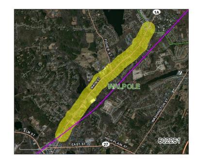
The proposed project consists of reconstructing 8,000 feet of Route 1A and includes improvements to the intersection and approaches at Fisher, Gould, North, Bullard/Willet Streets, and the Stop and Shop Plaza. The Route 1A bridge over the Neponset River, near the intersection with North Street, will be analyzed to determine if it can be rehabilitated or if it requires replacement. The limits of work are from approximately 2,000 feet north of Route 27 north to the Norwood town line.
