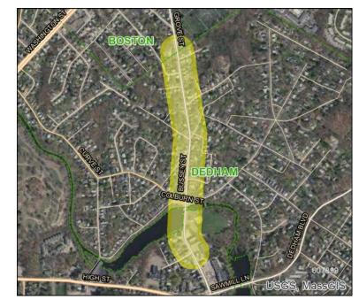
Improvements along the Bussey Street corridor will include resetting and setting the curb and reconstructing ADA compliant sidewalks and ramps on both sides of the roadway. Some pavement reconstruction may be necessary to obtain the necessary curb reveal. Minor geometric improvements at the intersection with Colburn Street and Clisby Avenue will make them more pedestrian friendly. Shared bicycle accommodations are planned.
