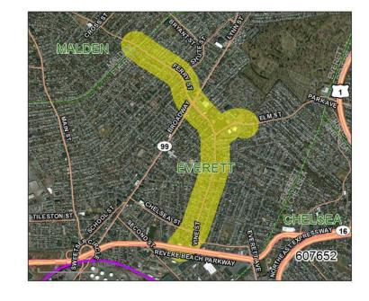
The project will reconstruct Ferry Street from the Malden city line (Belmont Street) to Route 16 and Elm Street between Ferry Street and Woodlawn Street. The work will include resurfacing and construction of new sidewalks, wheelchair ramps, and curb extensions. The traffic signals at five locations and the fire station will be upgraded. The signalized intersection at Chelsea Street will be replaced by a roundabout.
