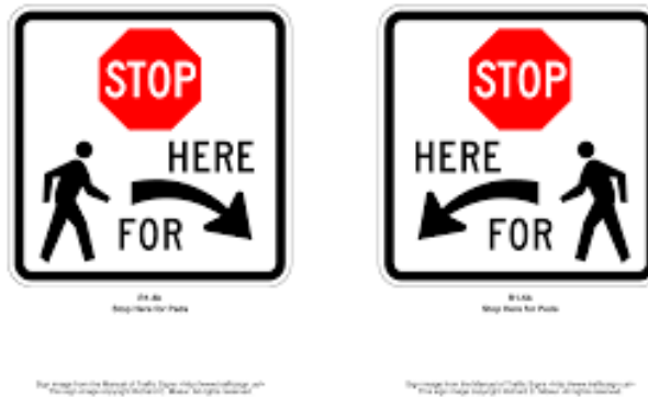
Figure 13 MUTCD Standard “Stop Here for Pedestrians” Sign
