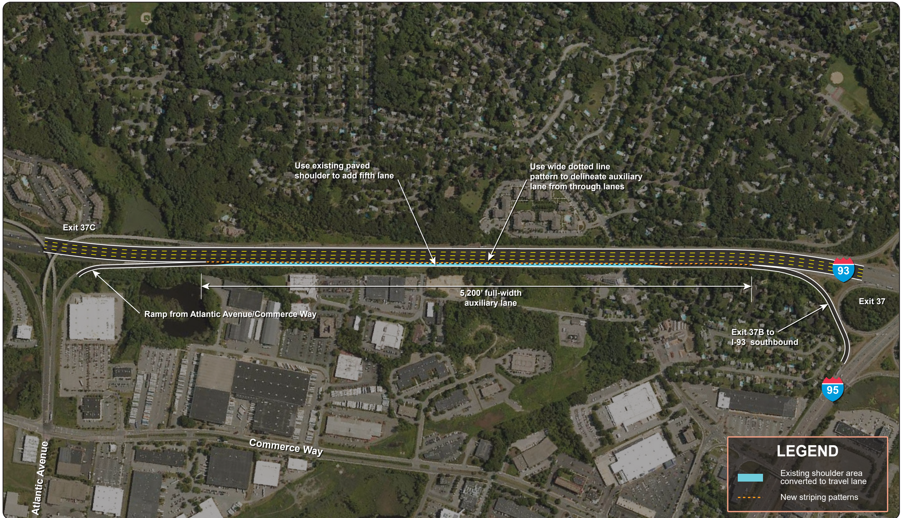
Figure 11 Location 2: I-93 Southbound Segment between Exit 37C (Commerce Way) and Exit 37B (I-95): Alternative 1—Create an Auxiliary Lane on I-93 Southbound
