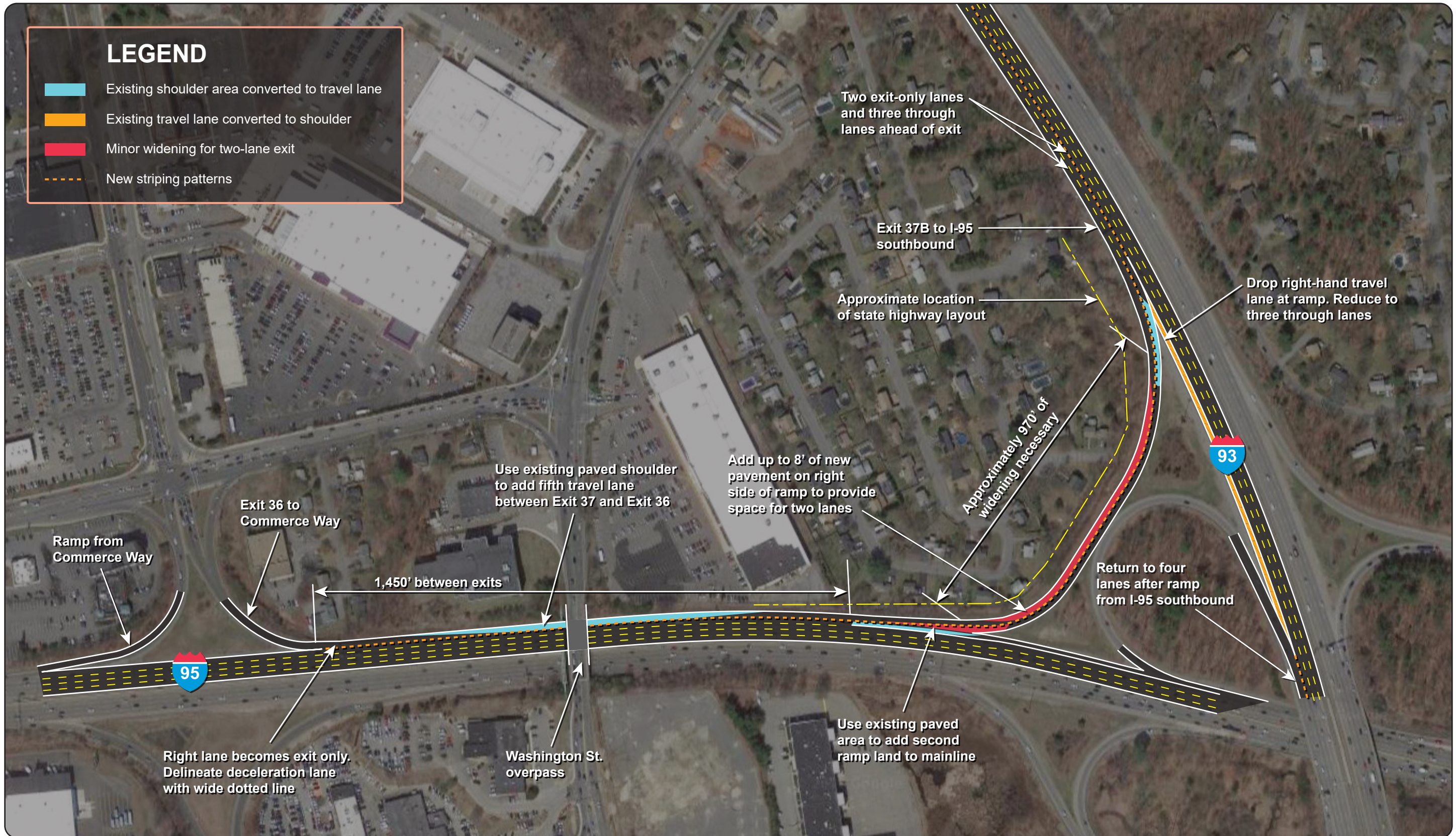
Figure 13 Location 2: I-93 Southbound Segment between Exit 37C (Commerce Way) and Exit 37B (I-95): Alternative 3—Two-lane Ramp at Exit 37B
