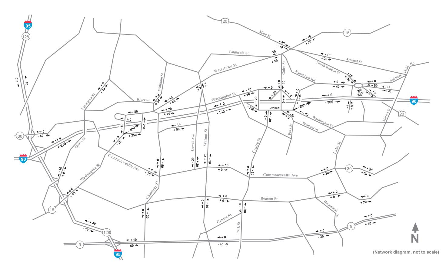
Figure 13: Alternative 4 - Projected 2030 AM Peak-Hour Traffic-Volume Changes from No-Build
