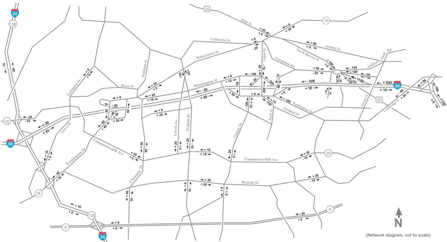
Figure 10: Alternative 2 - Projected 2030 PM Peak-Hour Traffic-Volume Changes from No-Build
