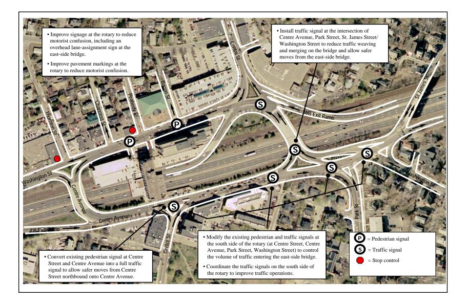
**Figure E-1: Improvements Tested in Alternative 5**
