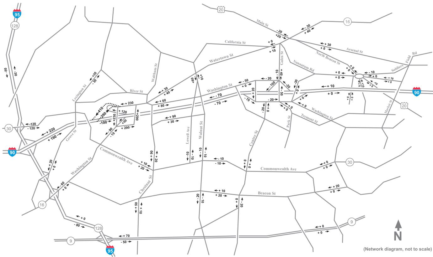
Figure 12: Alternative 3 - Projected 2030 PM Peak-Hour Traffic-Volume Changes from No-Build
