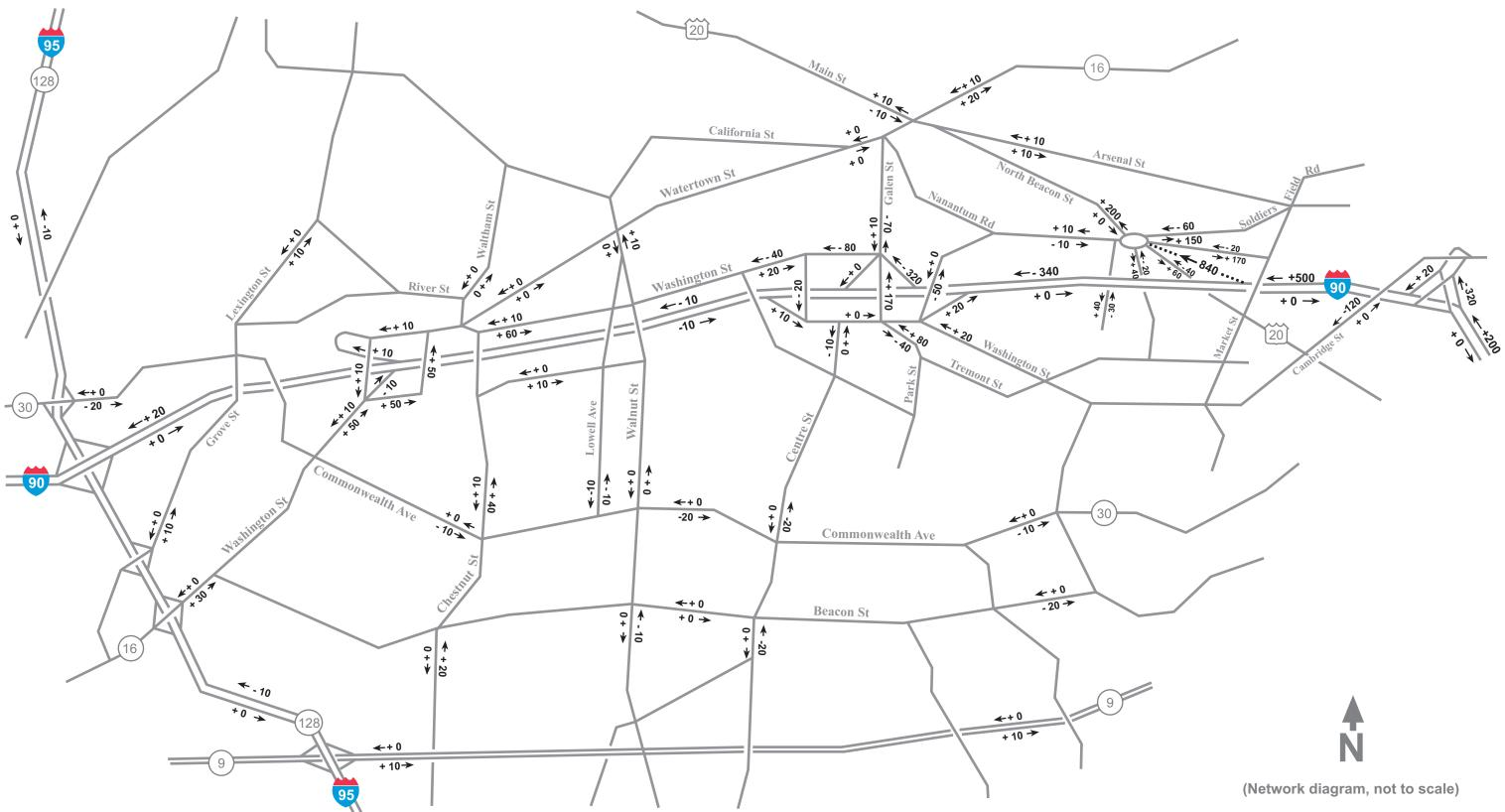
Figure 9: Alternative 2 - Projected 2030 AM Peak-Hour Traffic-Volume Changes from No-Build
